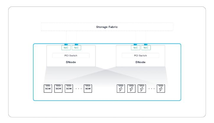
As you can see in the figure above, each HA Enclosure houses two DNodes that are responsible for routing NVMe-oF requests from their fabric ports to the enclosure's SSDs through a complex of PCIe switch chips on each DNode.
