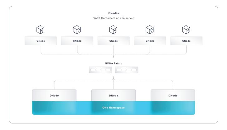
From the key points and diagram above, you've probably figured out that the DASE architecture is based on two basic components: CNodes run that run all the software and DBoxes that hold all the storage media, and system state.
