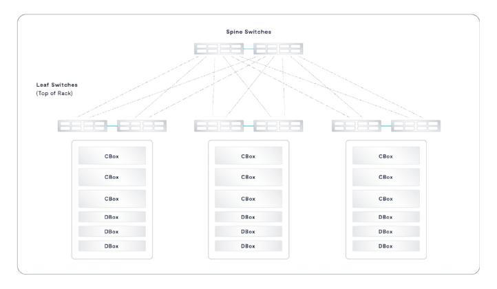
Leaf-spine networking allows DASE clusters to grow to well over 100 appliances, especially when large port count director class switches are used in the spine. Planning is underway for very large clusters of 1,000 appliances or more, so the groundwork will be laid before customers reach that size.
