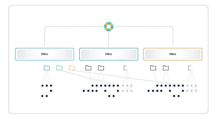
VAST Servers load the 1 GB consistent hash table into memory at boot. When a VAST Server wants to find data within a particular file or object, it calculates the hash of the element's handle, and performs a high-speed memory lookup to find which enclosure(s) hold that element's metadata by hash range. The VAST Server can then read the element's V-Tree from one of the DBoxes responsible for that portion of the hash space.
