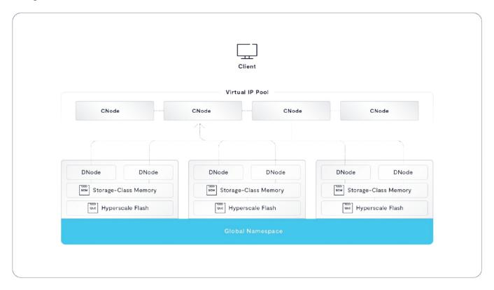
When the data in a cluster's write buffer reaches a high water mark, the system starts the process of migrating data from the SCM to hyperscale flash. The migration process is distributed across multiple CNodes in parallel.
