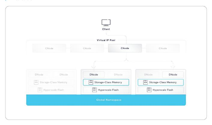
When a client writes data to an Element in the VAST DataStore, the CNode receiving that request writes the data to write buffers on two SCM SSDs. If encryption at rest is enabled, the data is encrypted by the CNode before being written.
