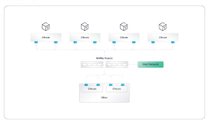
The Connect via Switch option runs the NVMe back-end fabric and the front-end host network connections as two VLANs on the NVMe fabric switches that are included in each DASE cluster. The customer's host network is connected to the cluster through an MLAG connection from the fabric switches to the customer's core switches as shown in green above.
