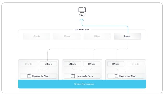
When a CNode receives a read request, that CNode locates the root of the metadata V-Tree for the Element being read using the cluster's consistent hash table. It then follows the V-Tree's pointers in SCM until it finds pointers to the requested content.
