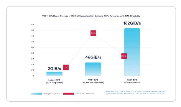
GPU Direct Storage also reduces the overhead of accessing storage. When we tested a VAST Cluster with an NVIDIA DGX-A100 GPU server, as shown in the chart above, the combination of NFS over RDMA and multipath load balancing across the DGX-A100's eight 200Gbps HDR InfiniBand boosted total bandwidth from the NFSoTCP's 2 GiB/s to 46 GiB/s. However, moving all that data through main memory to the GPUs eats up half the DGX-A100's 128 AMD ROME cores.
