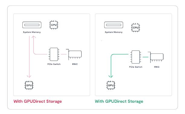
NVIDIA's GPUDirect Storage provides a direct RDMA path for NFS data from an RNIC into the memory of a GPU, thus bypassing the CPU and the CPU's memory. GPU Direct Storage (GDS) vastly increases the amount of data GPUs can access by eliminating the main memory-to-GPU bandwidth bottleneck of 50 GB/s. Using GDS the server can transfer data into the GPU from multiple RNICs in parallel, boosting total bandwidth to as much as 200 GB/s.
